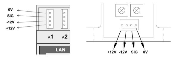
A typical sensor cable will be assembled as follows:
